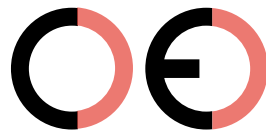
False CE Mark (too far)
